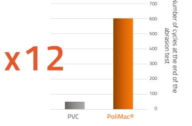
ASTM A975-21 (Section 13.1.5) –"Standard Specification for Double-Twisted Hexagonal Mesh Gabions and Revet Mattresses (Metallic-Coated Steel Wire or Metallic-Coated Steel Wire With Poly(Vinyl Chloride) (PVC) Coating)"
